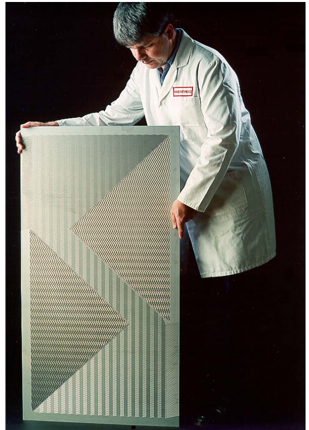
Figure 18: An etched PCHE lamination (Courtesy of Heatic Ltd, Poole, UK).
