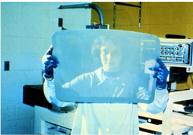
Figure 6: Low resolution TV shadow aperture mask (Courtesy of PCMI).
